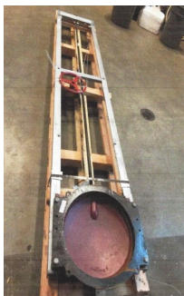
Figure 1 - New sluice gate
